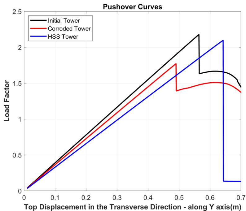
Figure 3.14: Pushover curves of the three versions of suspension transmission towers
